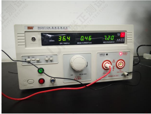
测试后耐压确认 After pressure test
